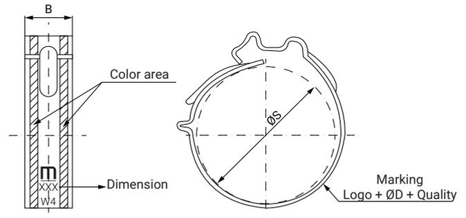
The Clip Clamp is manufactured entirely from one strip of stainless steel.
